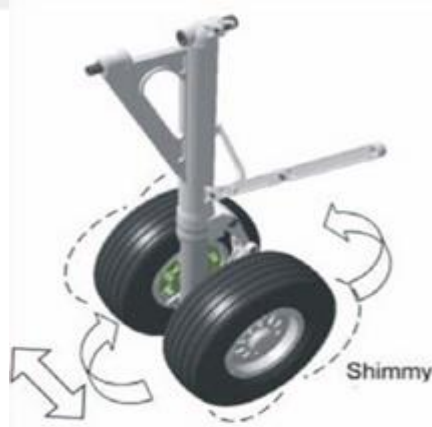
Figure 3.32 : 2 DOF (Yaw and lateral) shimmy model [21].
