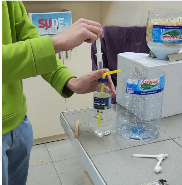
Figure 3.6 Water Pump Design with Syringe
