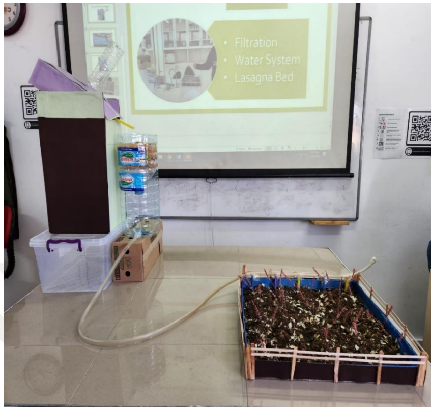
Figure 3.7 Prototype of Drip Irrigation System
