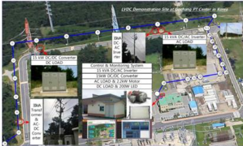
Figure 4.10 : Topology of the LVDC Network Test Site [64]
