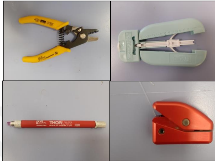
Figure 7: Jonard JIC-375 on the upper left, MicroStrip 0.010 on the upper right, diamond cutter (Thorlabs S90R on the bottom left, holder (Thorlabs BFT1) bottom right
