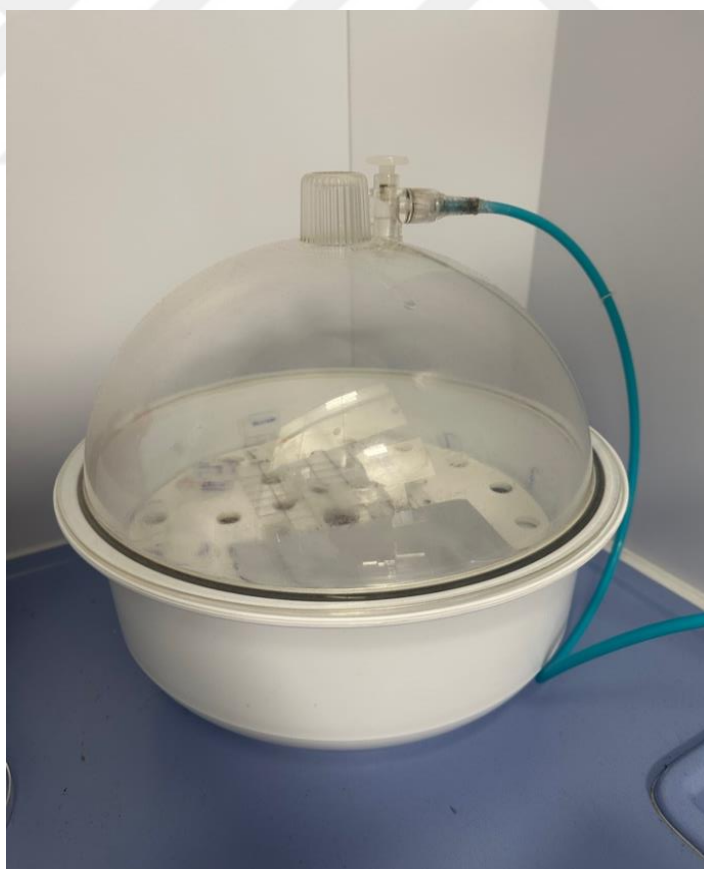
Figure 19: Desiccator device found in our laboratory used for primary drying process of reagent.
