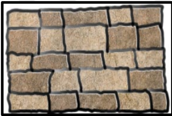
Figure 3.6. Coursed rubble masonry exterior view
