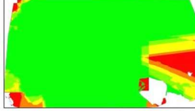
Figure 4: Number of overlapping images computed for each pixel of the orthomosaic. Red and yellow areas indicate low overlap for which poor results may be generated. Green areas indicate an overlap of over 5 images for every pixel. Good quality results will be generated as long as the number of keypoint matches is also sufficient for these areas (see Figure 5 for keypoint matches).
