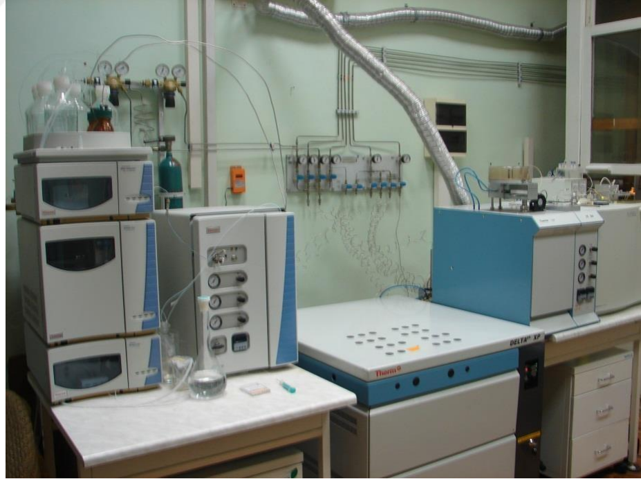
Şekil 3.13. Kararlı İzotop Spektrometresi - Delta-PlusXP; Thermo Fisher Scientific, Waltham, MA, ABD.
