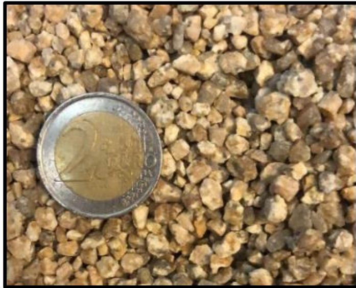
Figure 4.5. The sand filling the hydrate cell
