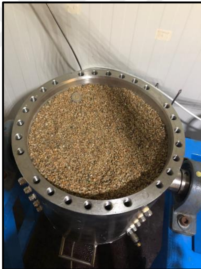
Figure 4.6. Hydrate cell filled with sand and water
