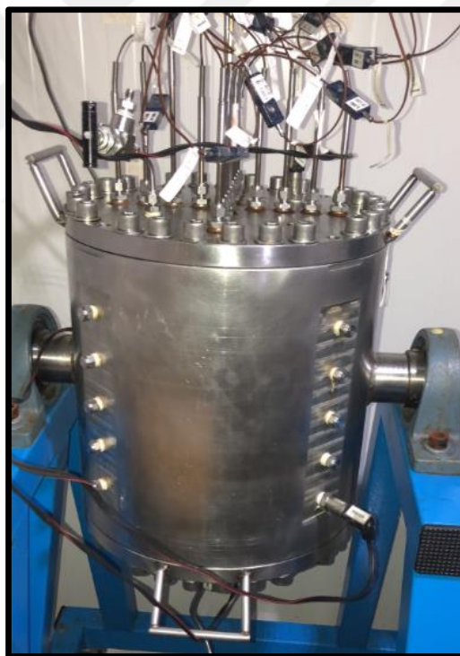
Figure 4.4. Cylindrical high pressure cell used for hydrate formation experiments
