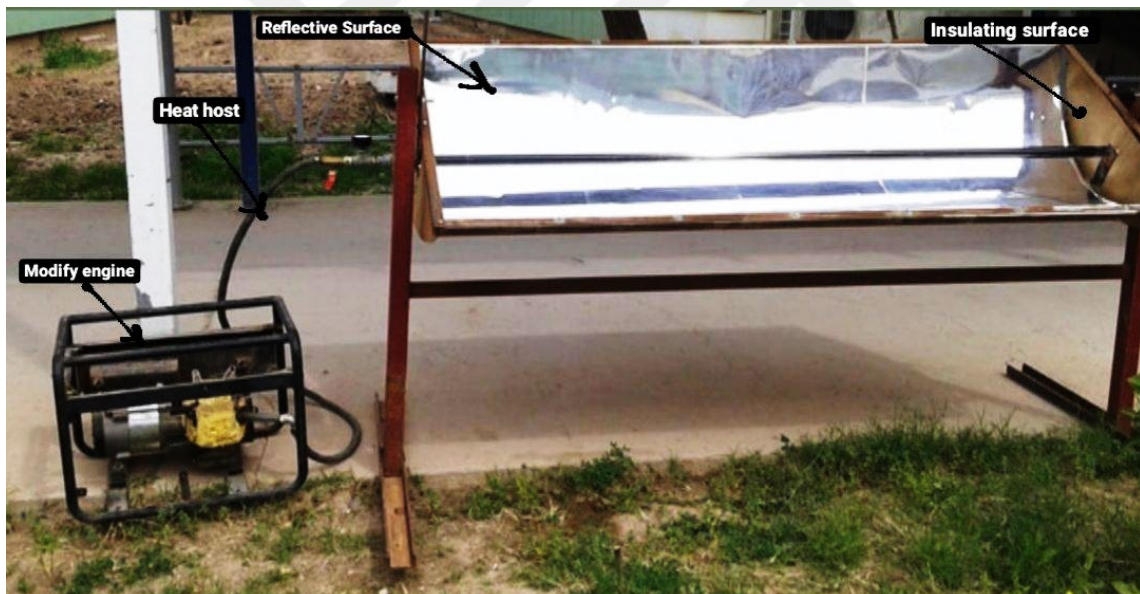
Figure 3.1: Solar collector with modify generator.
