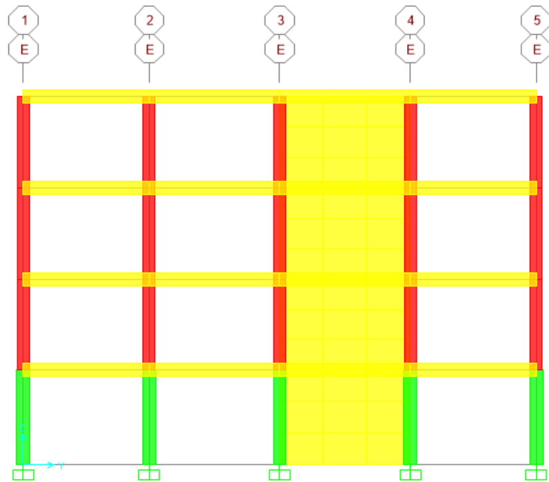
Figure 4.2. Shear-walls of stairs which cause to a small eccentricity to y-direction
