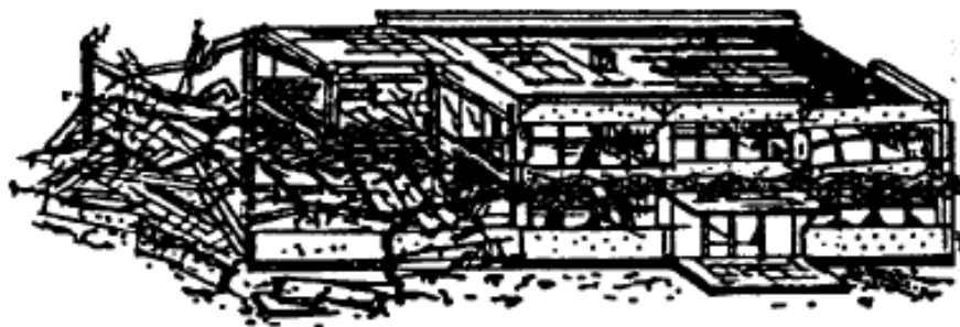
Figure 3.10. Collapse damage level of a structure (EMS-98)
