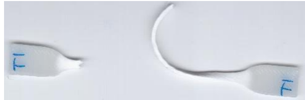
Figure 2.9. Fractured TPU tensile test specimen after the uniaxial tensile test.
