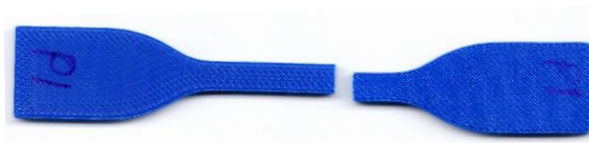
Figure 2.8. Fractured PLA tensile test specimen after the uniaxial tensile test.
