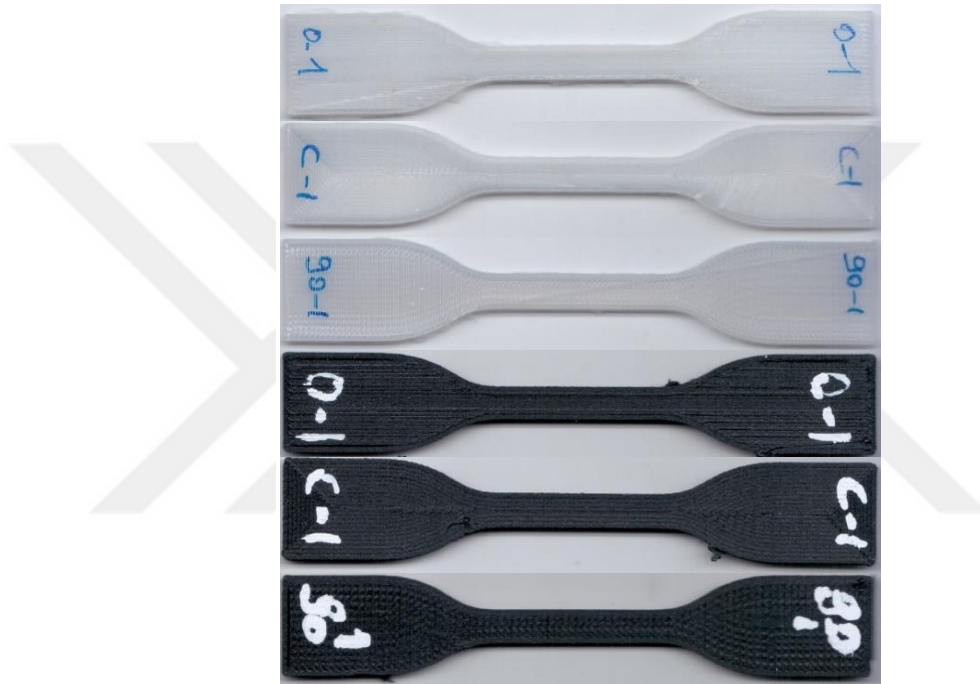
Figure 3.1. Tensile test specimens printed with PA and PAHT CF15 filament and having 0°, 90° raster angles, and a concentric infill
