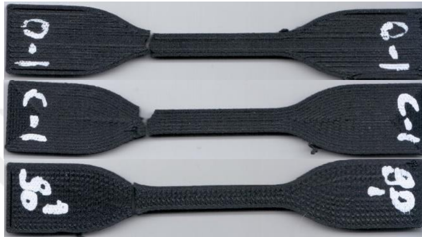
Figure 3.9. The fractured tensile test specimens printed with PAHT CF15 and having 0°, 90° raster angles, and a concentric infill.
