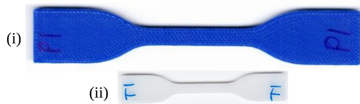
Figure 2.3. 3D printed PLA and TPU dogbone specimens. (i) PLA specimen was printed using Ultrafuse blue PLA filament, and the. (ii) TPU specimen was printed using Ultrafuse TPU 85A filament. The P in the naming indicates that the material is PLA, and T indicates that the material is TPU.
