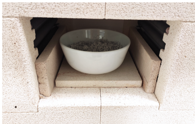
Figure 14 The photograph of the sample in Nüve muffle furnace before the heat treatment
