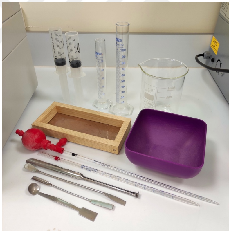
Figure 12 At the back side, from left to right; the photo of molds with piston, 50 ml and 100 ml of graduated cylinders, 1000 ml of beaker. In the front side, from left to right; a wooden mold, vessel (with purple color), glass pipettes and spoons
