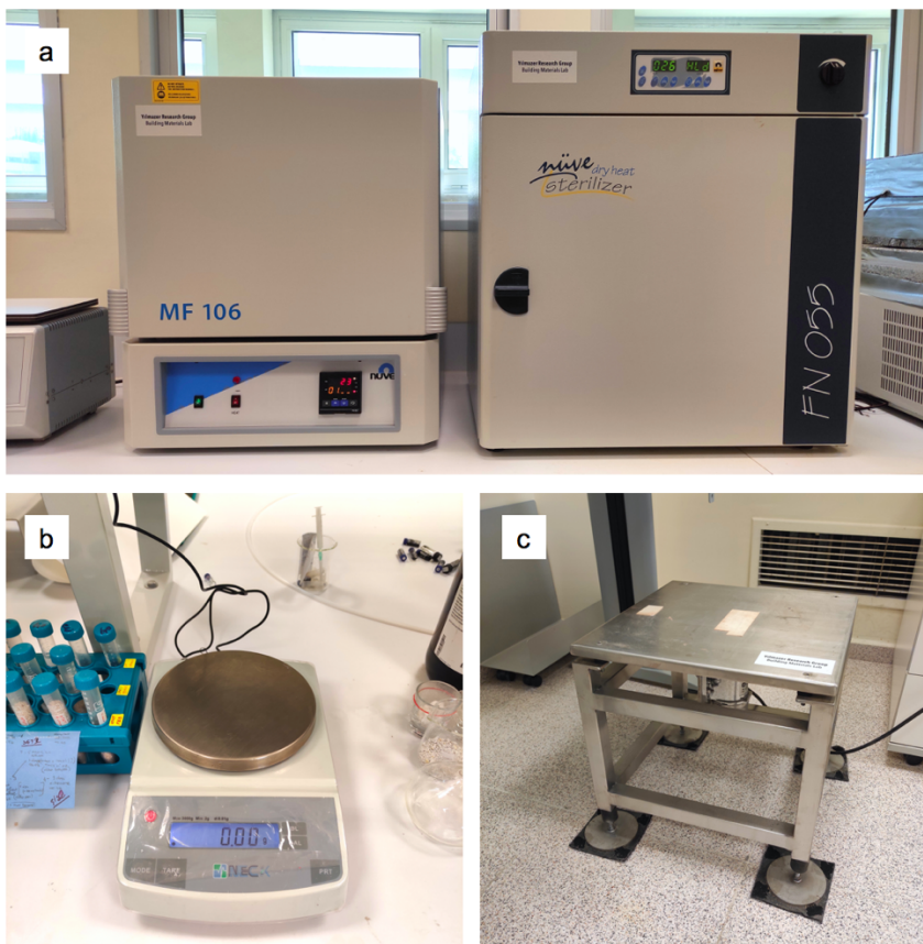
Figure 11 The photos of (a) Nuve muffle furnace (left) and Nuve dry air sterilizer oven (right), (b) precision balance and (c) vibrator
