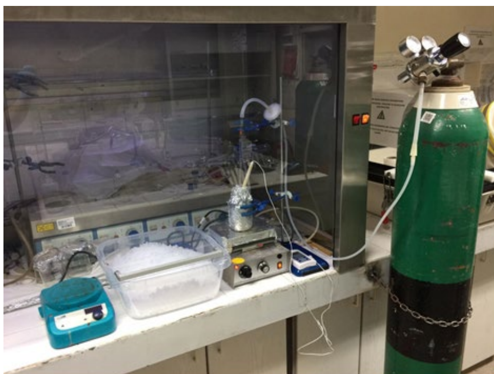
Figure 3.2. Setup for the hyperthermophilic electro-active archaea growth medium (ferric citrate solution) preparation
