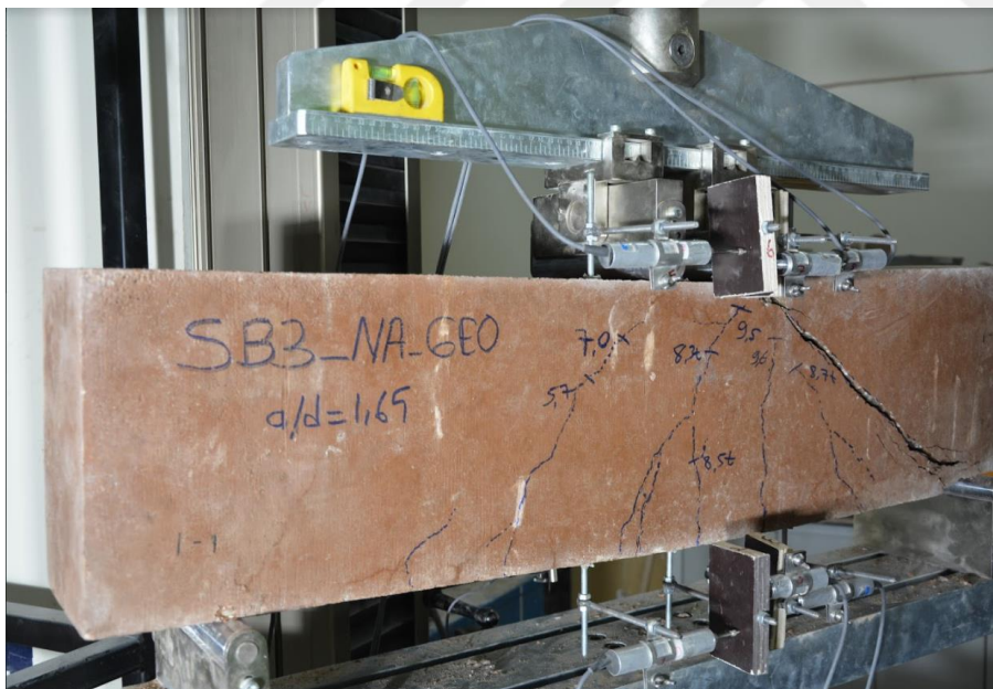
Figure 4.18 Growth of the cracks at the fron of the specimen
