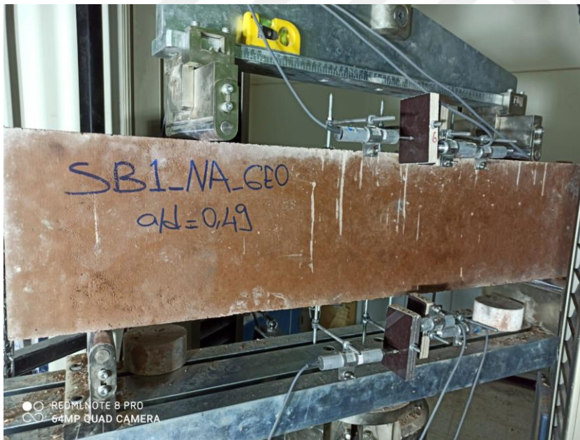
Figure 4.6 The image of the Shear-Critical Geopolymer Beam #1 during the experiment
