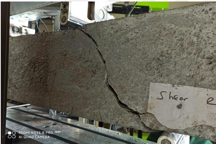
Figure 4.35 Shear crack between the upper and lower support
