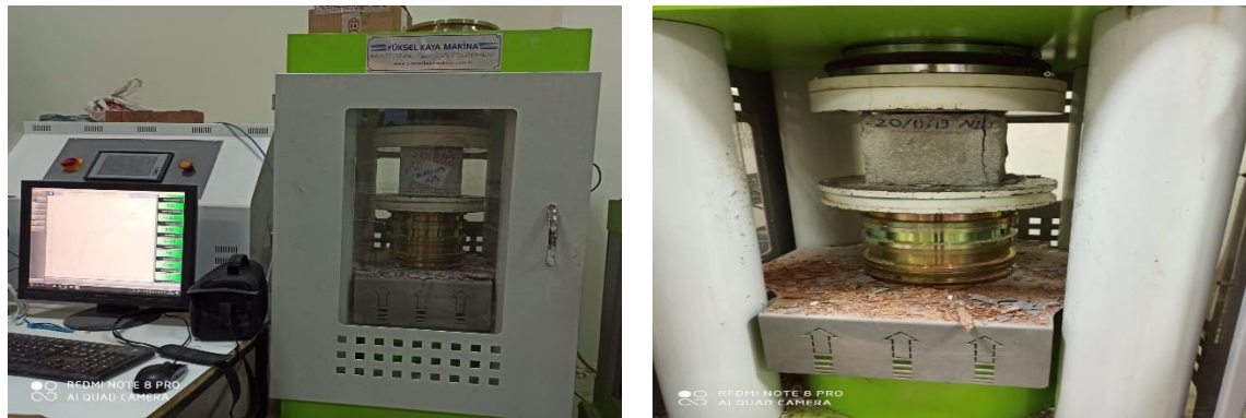
Figure 4.22 Compressive Strength Experiment of Concrete
