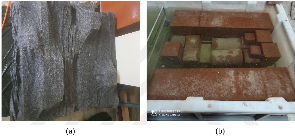
Figure 3.11. Curing of the specimens, (a) concrete samples, (b) geopolymer samples
