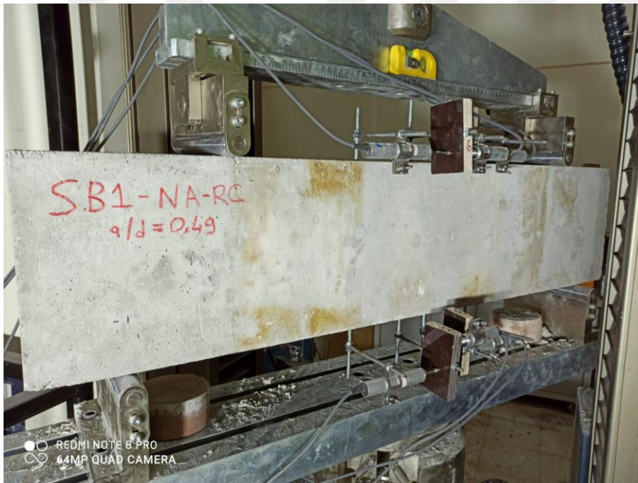
Figure 4.26 The image of the Shear-Critical Concrete Beam #1 during the experiment
