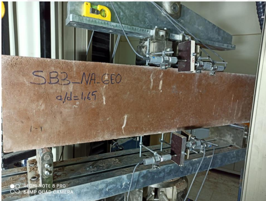
Figure 4.16 The image of the Shear-Critical Geopolymer Beam #3 during the experiment
