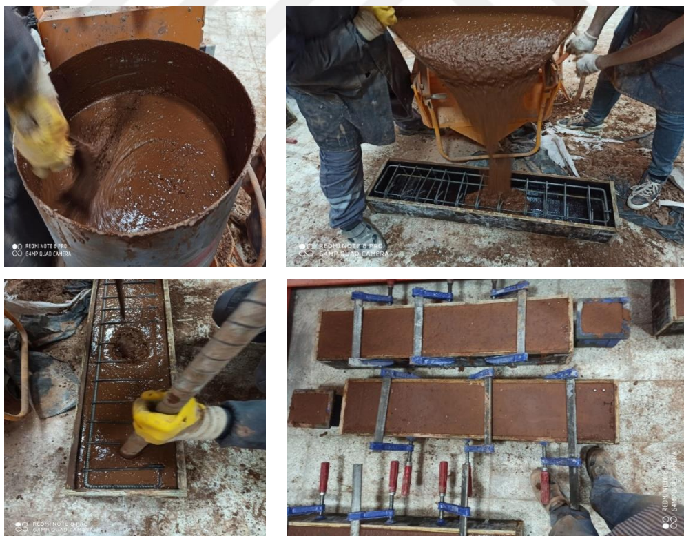
Figure 3.10. Casting and placing process of geopolymer mixtures
