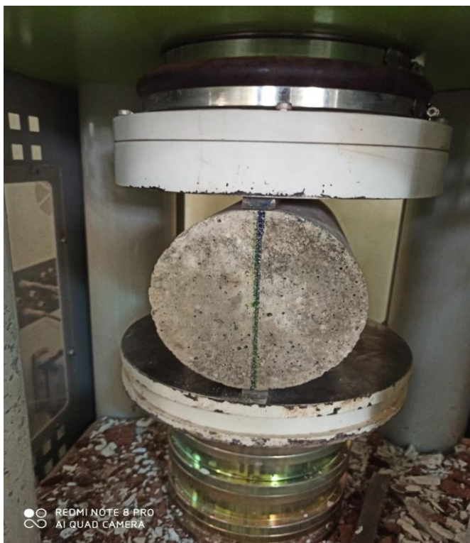
Figure 4.23 Splitting-Tensile Strength of Concrete
