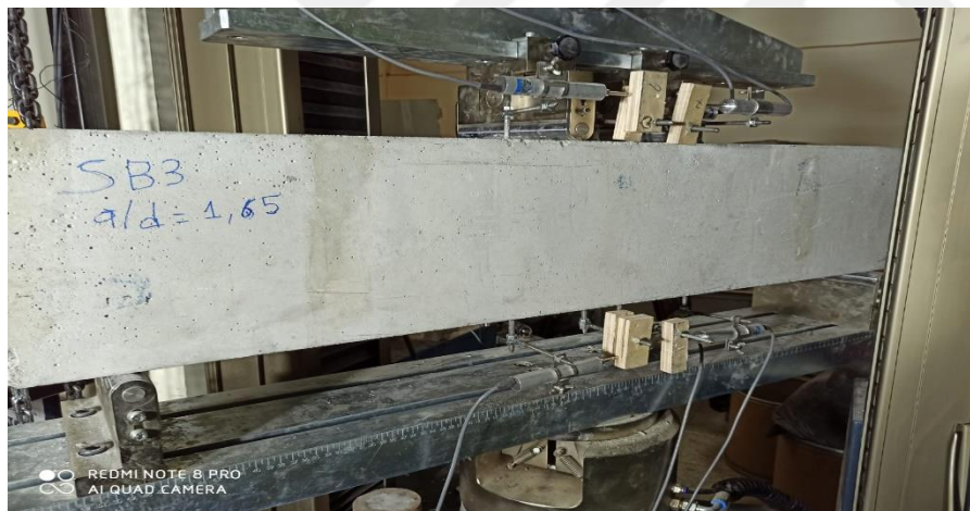
Figure 4.38 The image of the Shear-Critical Concrete Beam #3 during the experiment
