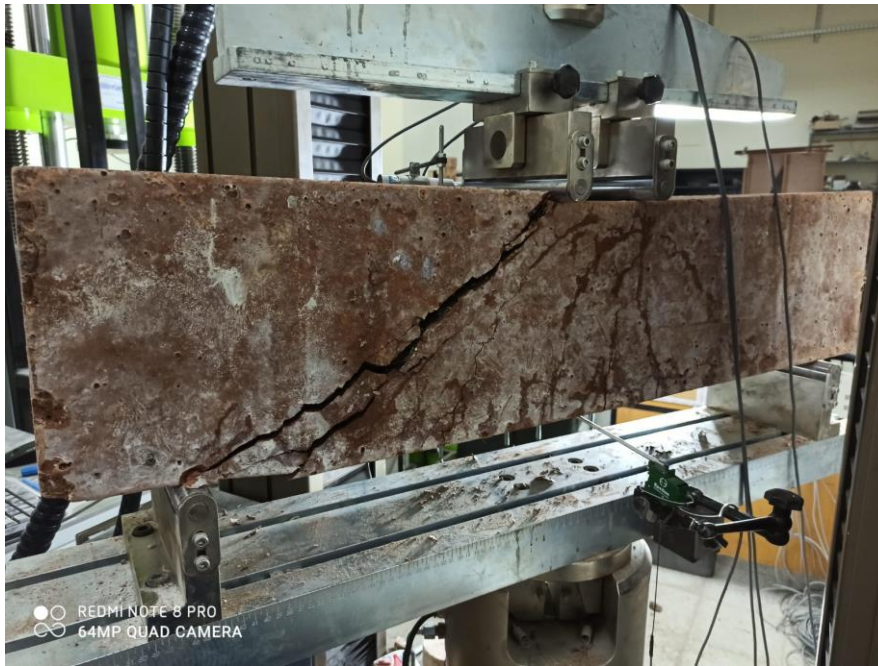
Figure 4.19 Large cracks at the back of the specimen after test
