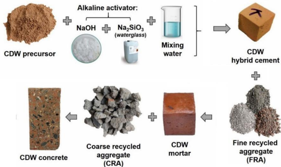
Figure 2.4. The process from CDW-based precursor to CDW-based concrete (adapater from Robayo-Salazar et al., 2020)
