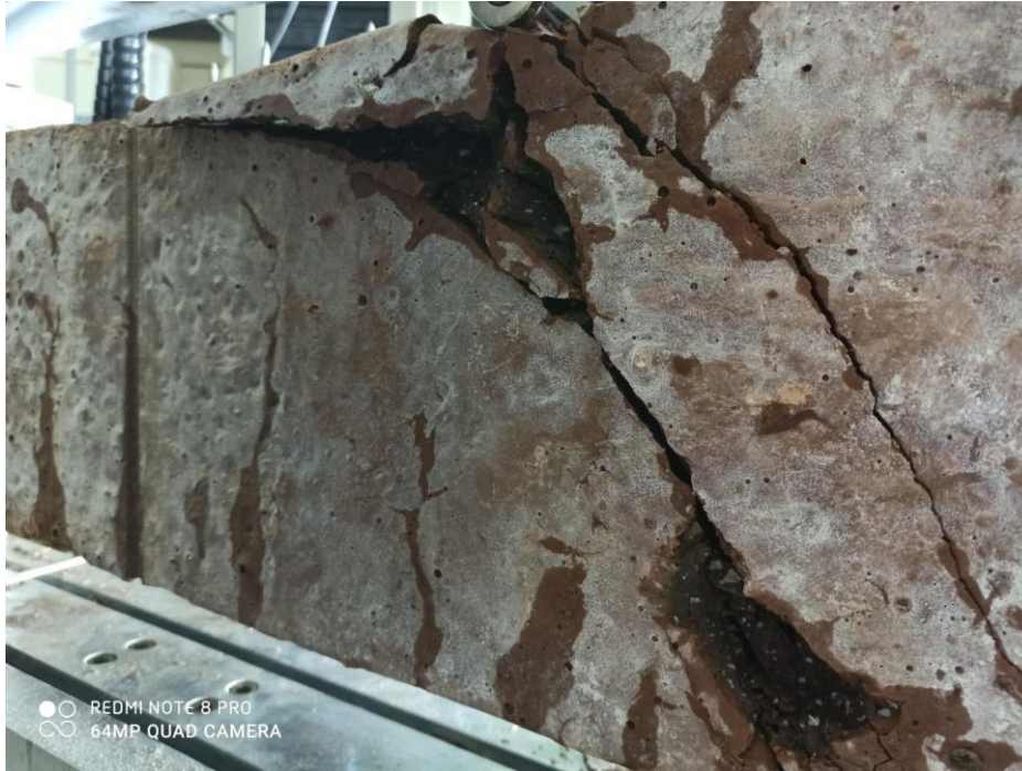
Figure 4.9 Large shear crack at the back of the specimen after the test
