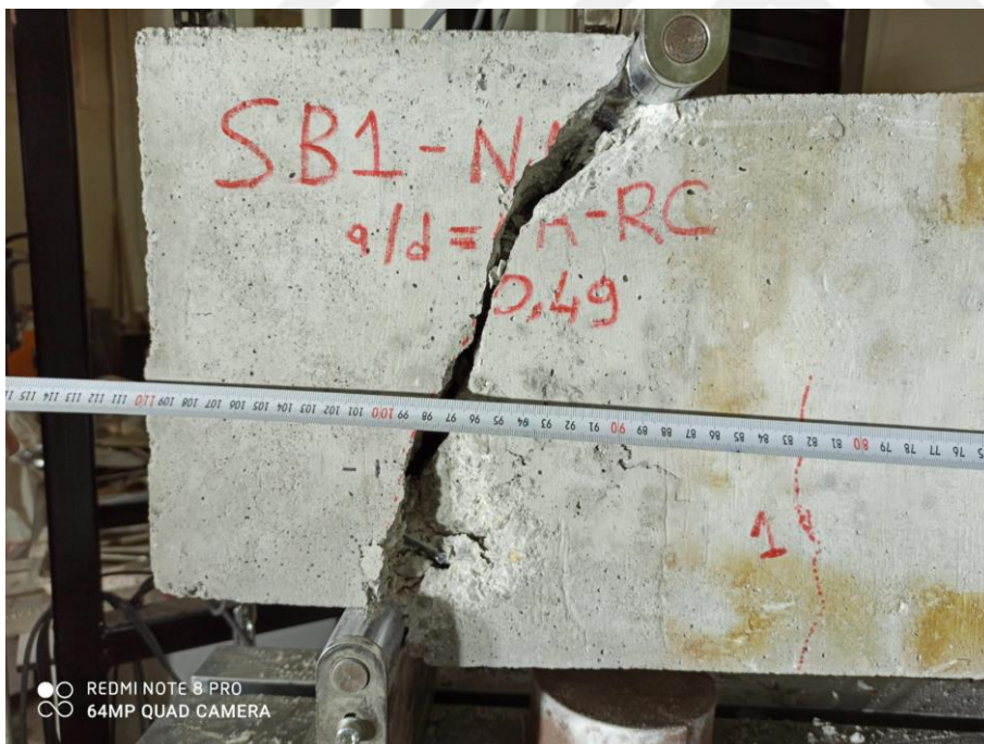
Figure 4.28 Growth of shear crack in the support area of the specimen
