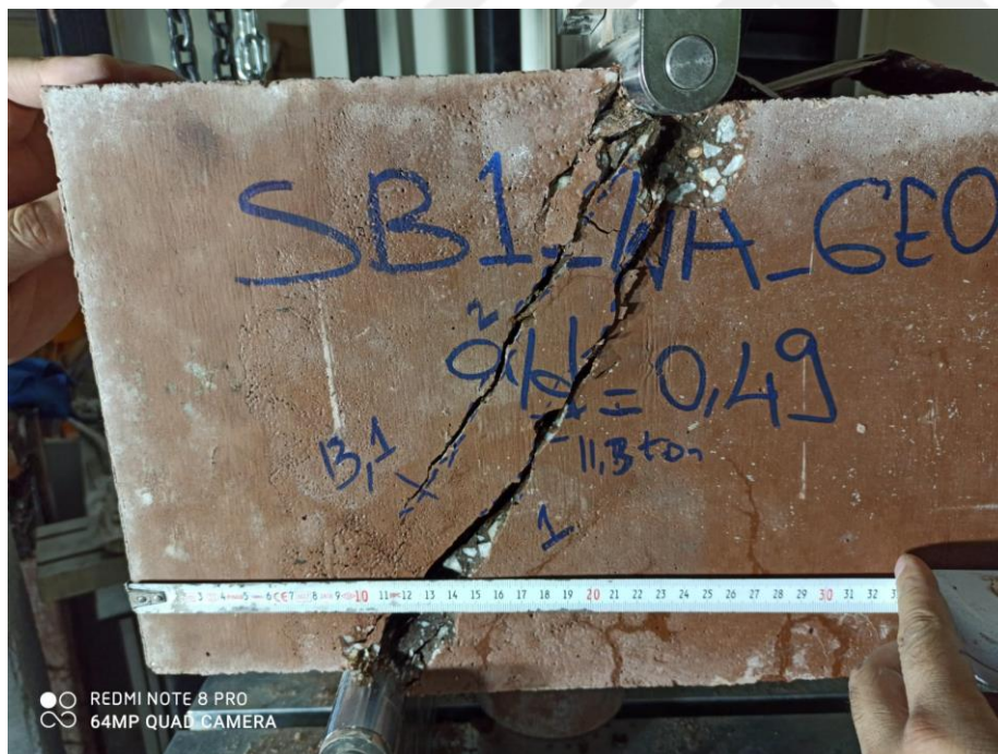
Figure 4.8 Growth of shear crack in the support area
