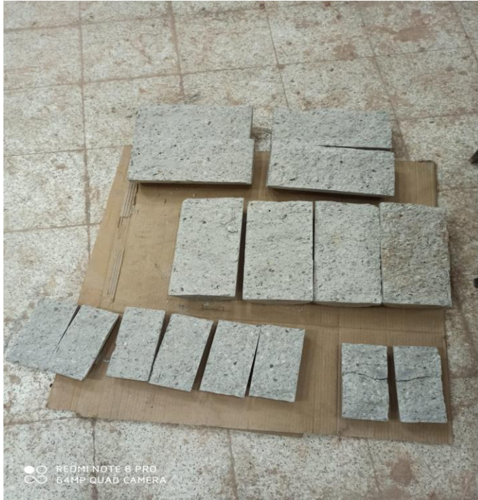
Figure 4.25 1 st and 2 nd group cylinders split into two after the experiment
