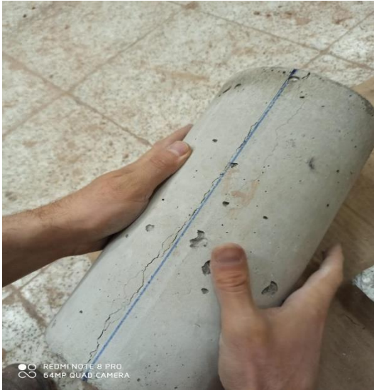
Figure 4.24 Crack formation in the cylinder after the test
