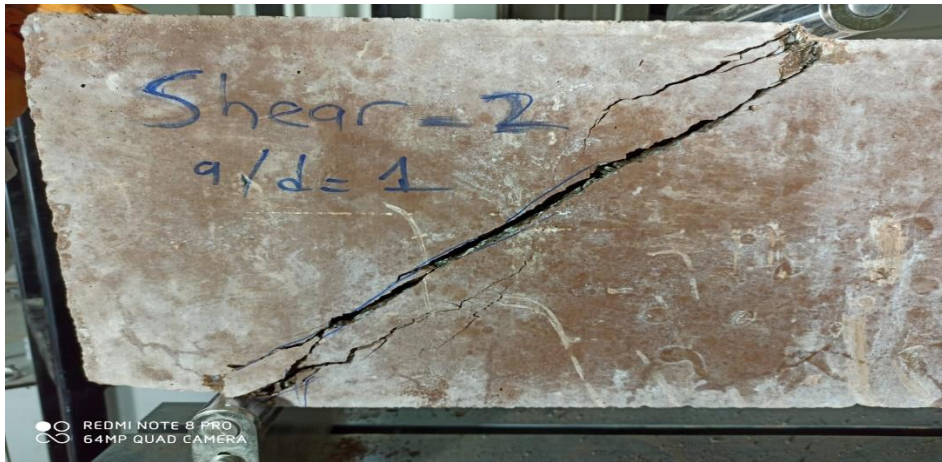
Figure 4.12 5 mm wide shear crack formation in the anterior between support
