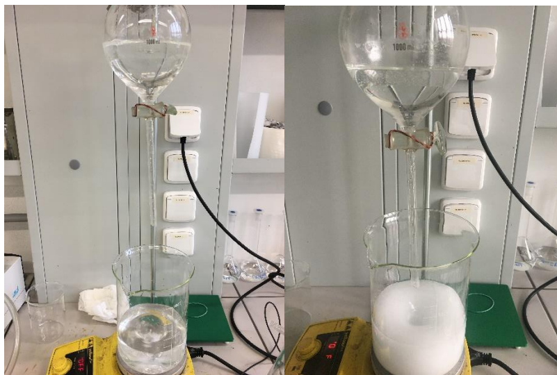
Figure 4. 5 a) Zinc nitrate hexahydrate, which has just begun to drip. b) The solution with the ZnO
