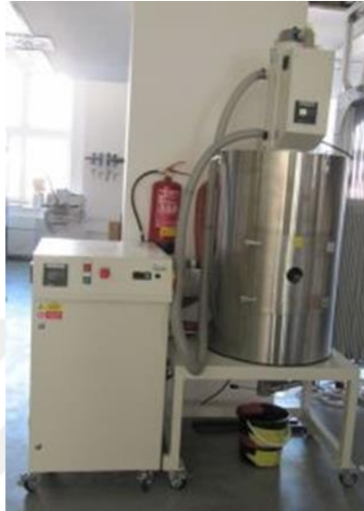
Figure 4. 9 Continuous drying system for hygroscopic materials
