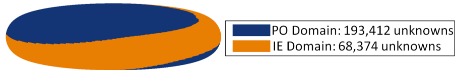
Figure 5.5: The region around the shadow boundary is chosen as the IE domain and the rest is chosen as the PO domain.
