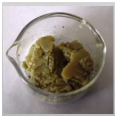
Figure 4.20 : A typical waxy product from FT synthesis by conventional catalyst.
