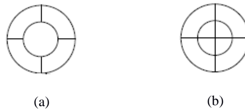
Figure 4.4 C-HOG filters: (a) C-HOG with a single circular central cell, (b) C-HOG whose central cell is divided into four angular sectors (Dalal and Triggs, 2005).
