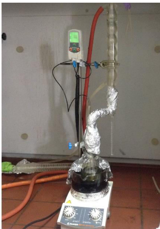
Figure 2.8 Dean Stark Apparatus.
