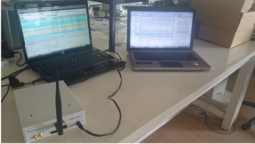
Figure 5.3: USRP test setup with receiver and transmitter in the Communication Laboratory at the METU EE Department.
