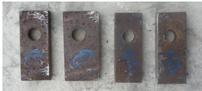
Figure 2.98. Filler plates of Specimen-7, after testing
