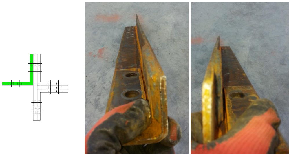
Figure 2.87. Bending on lower main member 1 (Specimen-6)
