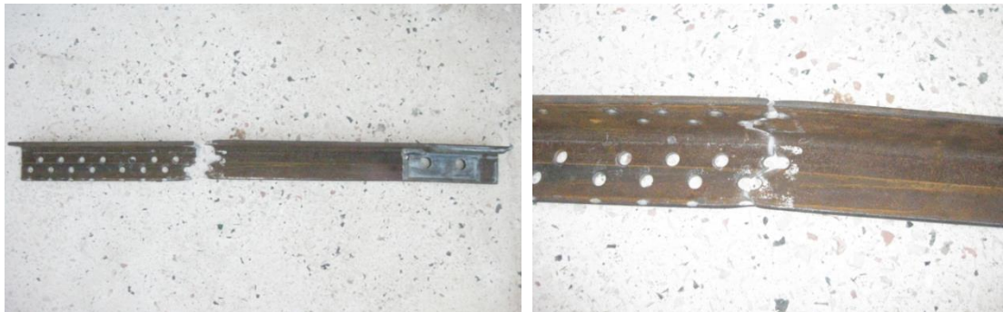
Figure 2.31. Deformations on ruptured angle member of Specimen-2
