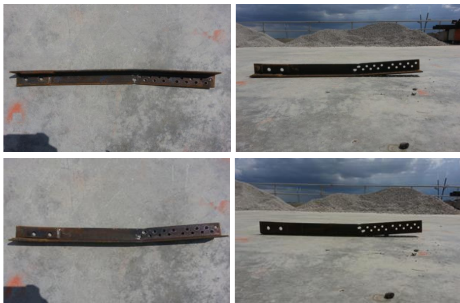
Figure 2.59. Bending of ruptured angle member of Specimen-4
