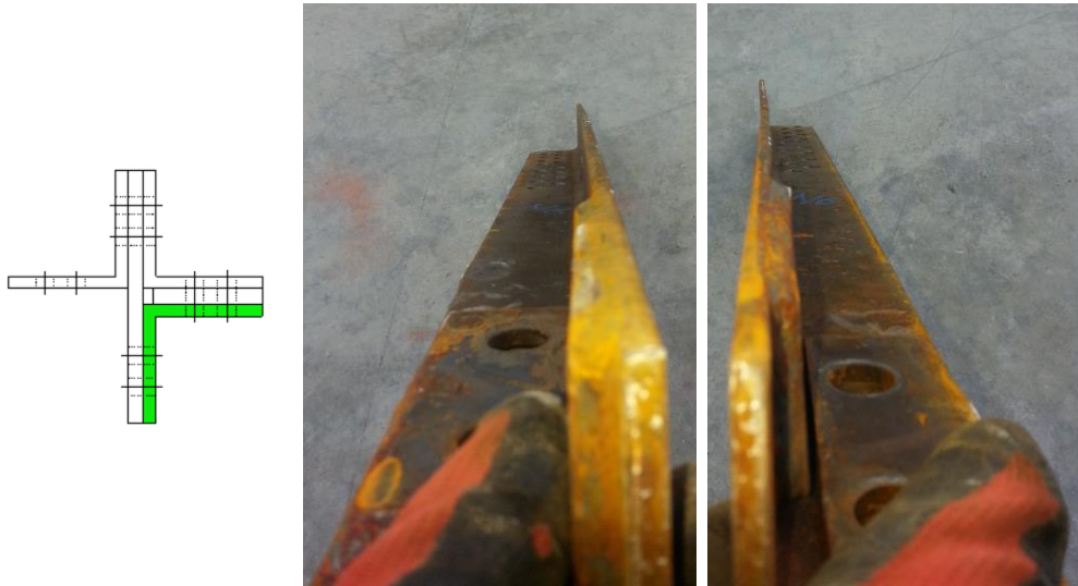
Figure 2.88. Bending on lower main member 2 (Specimen-6)
