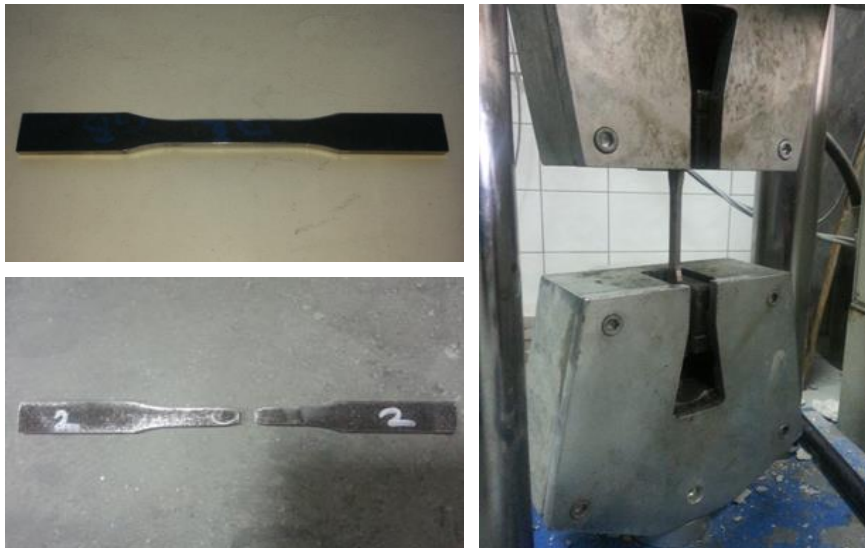
Figure 2.9. Tension test coupons and testing procedure
