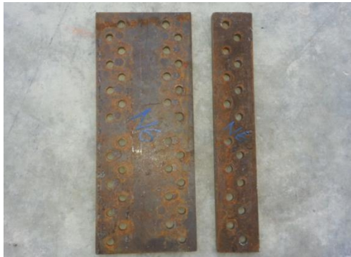
Figure 2.86. Filler plates of Specimen-6, after testing
