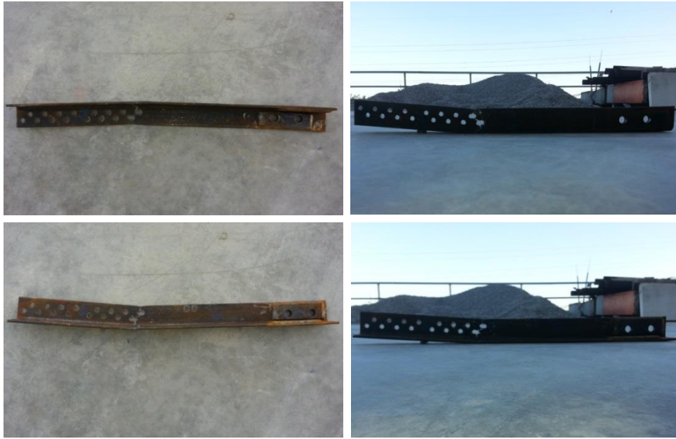
Figure 2.85. Bending of ruptured main member of Specimen-6
