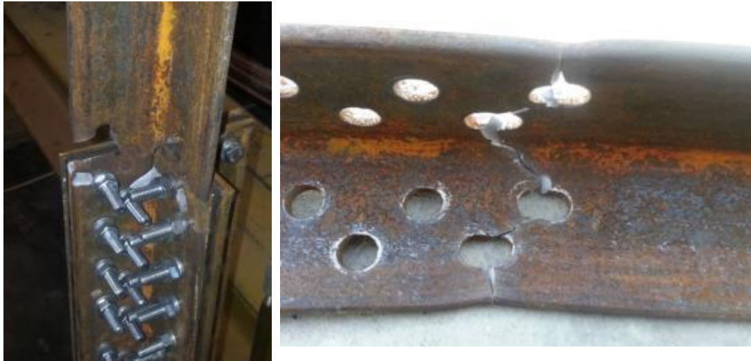
Figure 2.49. Rupture on critical path of Specimen-3
