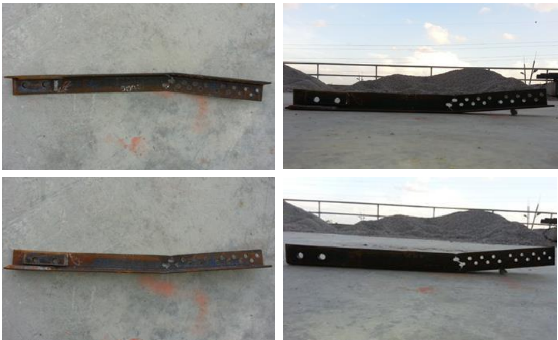
Figure 2.73. Bending of ruptured angle member of Specimen-5
