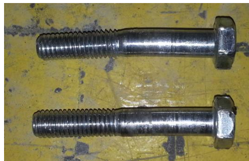
Figure 2.82. Bending deformation on bolts (Specimen-6)
