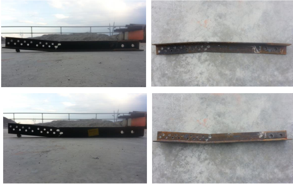
Figure 2.97. Bending of ruptured main member of Specimen-7
