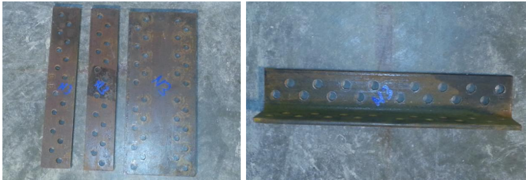
Figure 2.51. Reinforcement angle member and filler plates of Specimen-3, after testing
