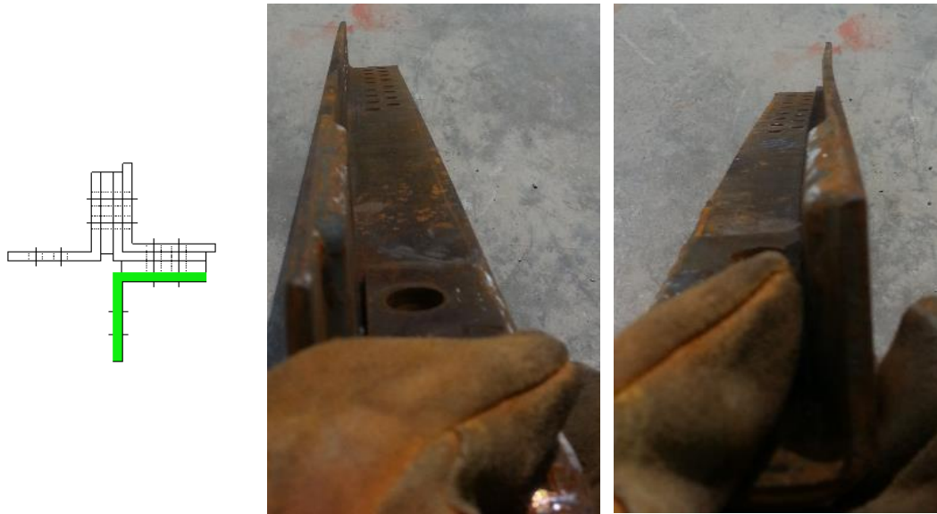
Figure 2.62. Bending on lower main member 2 (Specimen-4)
