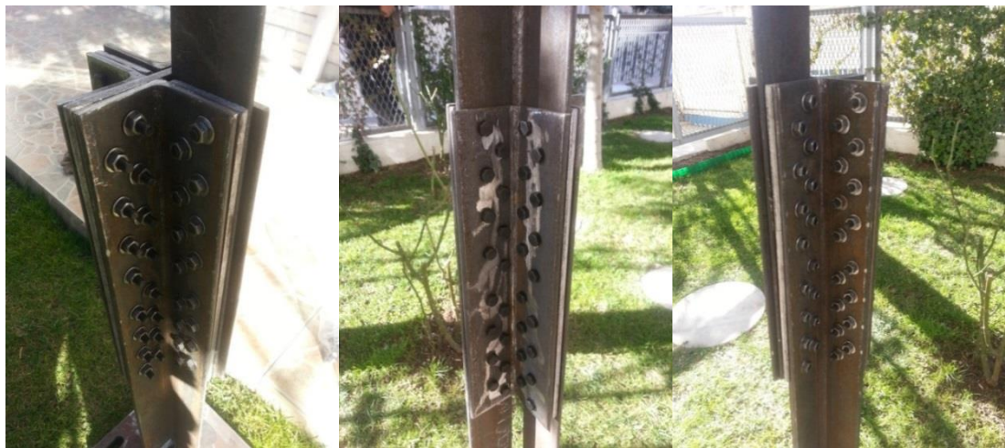
Figure 2.13. Members and connection detail of Specimen-1
