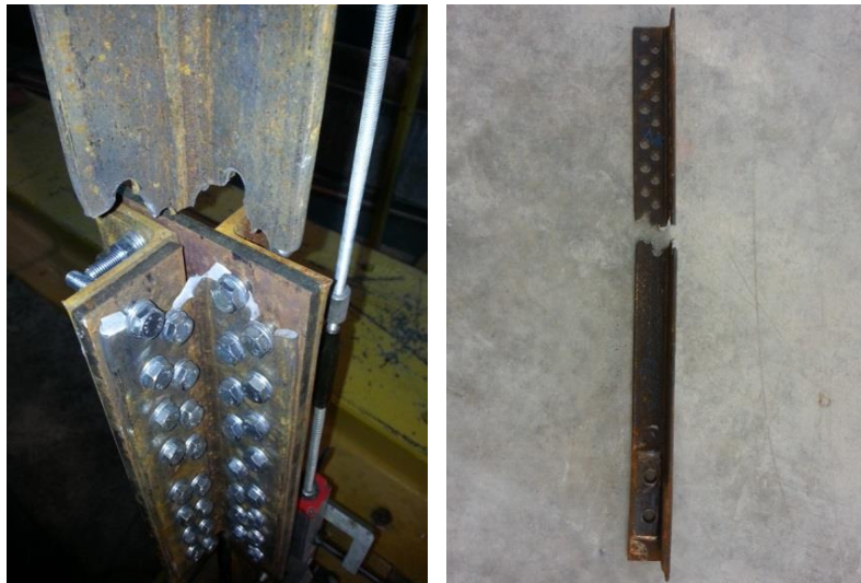
Figure 2.83. Rupture on critical path of Specimen-6
