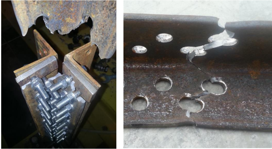
Figure 2.95. Rupture on critical path of Specimen-7
