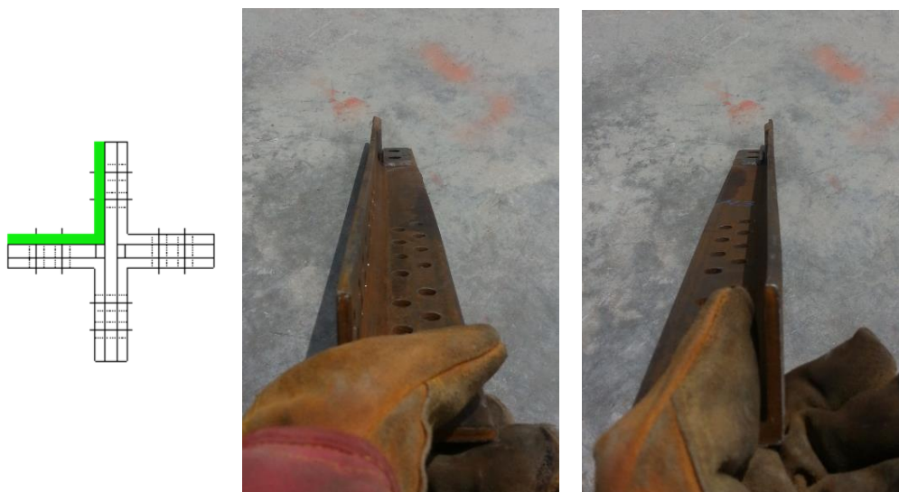
Figure 2.52. Bending on lower main member 1 (Specimen-3)
