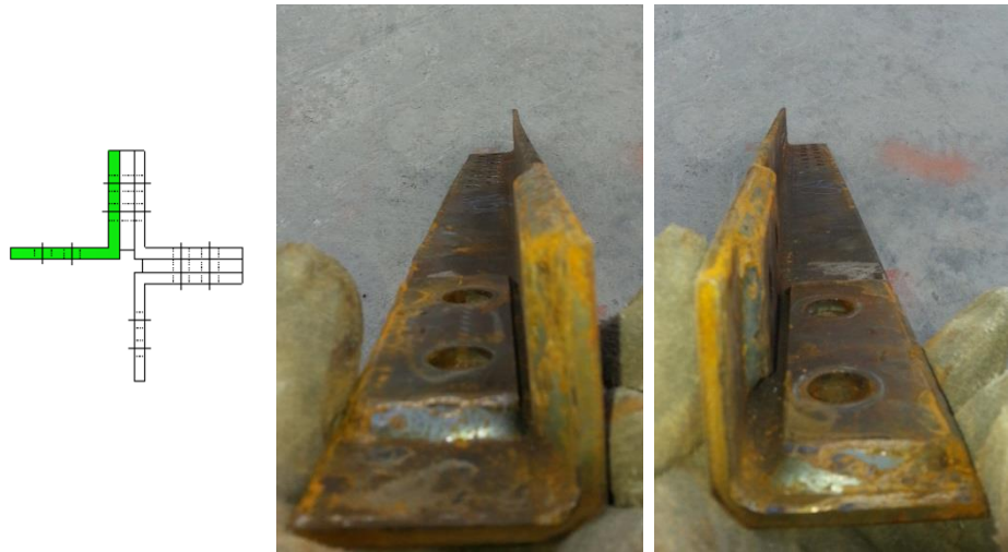
Figure 2.75. Bending on lower main member 1 (Specimen-5)
