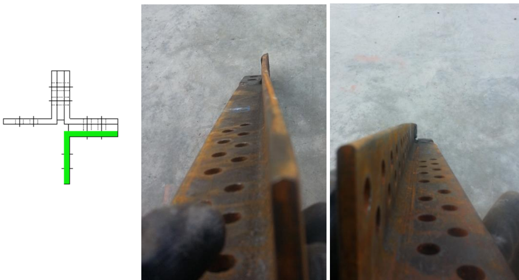
Figure 2.99. Bending on lower main member 2 (Specimen-7)
