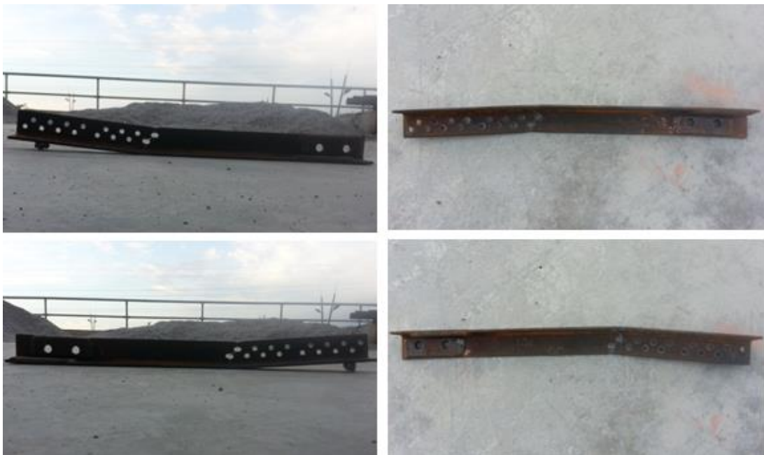
Figure 2.50. Bending of ruptured angle member of Specimen-3
