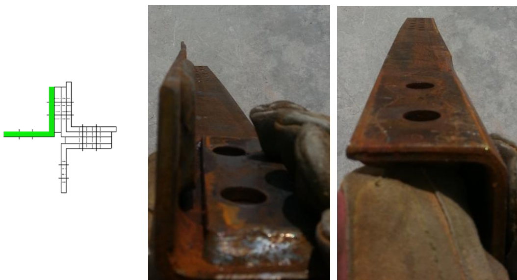
Figure 2.61. Bending on lower main member 1 (Specimen-4)
