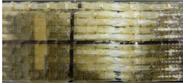
Figure 7.5. Tensile failure region in x-yarn direction (2 layers, plain weave, 5.85 x-yarns/layer/cm composite manufactured at 75 kPa vacuums)
