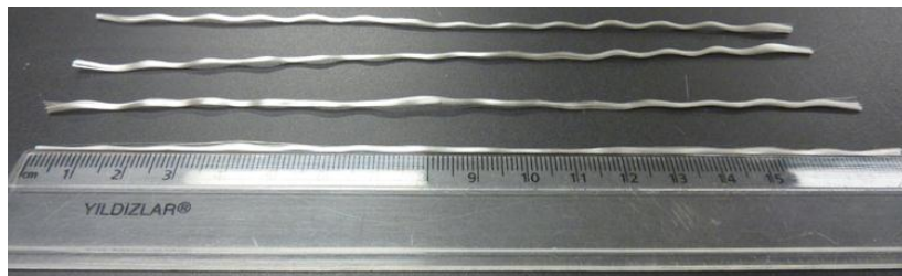
Figure 5.8. Z-yarn crimp measurement
