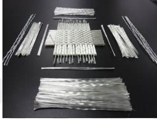
Figure 5.7. Separation of constituent yarns of dry preform
