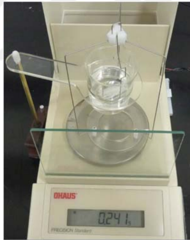
Figure 5.6. Density kit for volume measurement of analytical specimens
