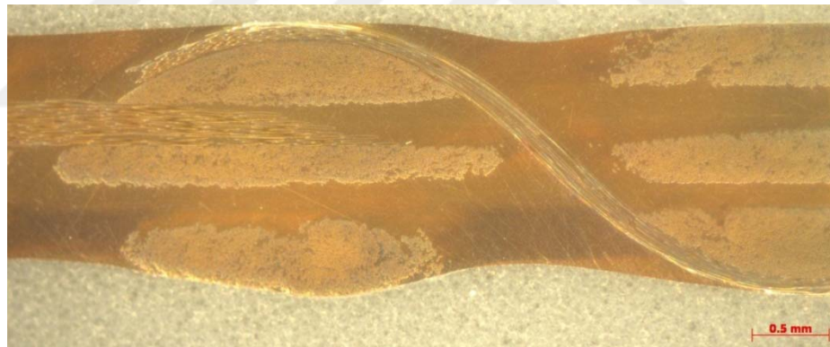
Figure 4.17. X-yarn cross section of 2 layers, plain weave, 4.87 x-yarns/layer/cm composite
