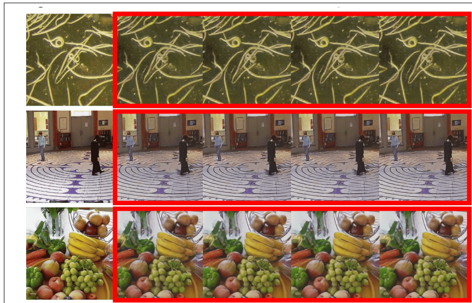
Figure 3.6. Qualitative results of image to image first stage model on train set (left column is original stimulus) (Images in red boxes represent 4 reconstructed sample images corresponding to the original stimulus on the left)
