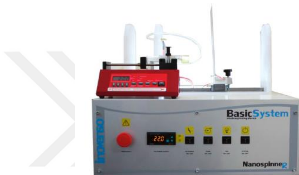
Figure 2.2 Nanospinner basic electrospinning unit (NanoSpinner 1 Electrospinning Equipment - Inovenso Inc. - PDF Catalogs | Technical Documentation | Brochure)
