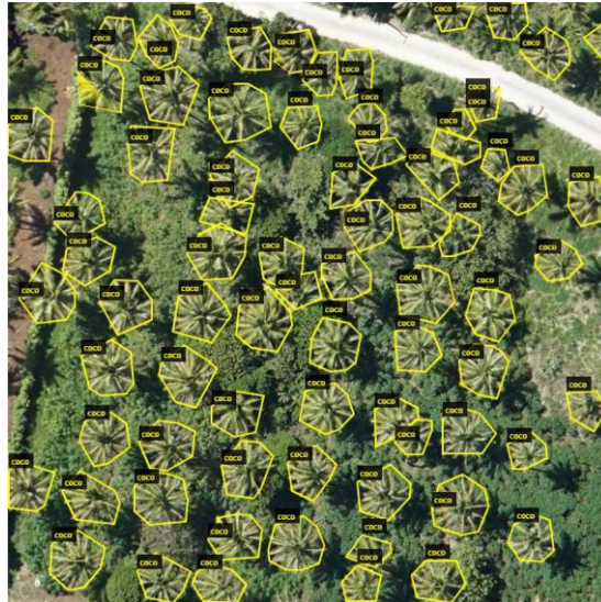
Figure 1.4 “Coconut trees, detection and segmentation in aerial imagery using mask region-based convolution neural network”
