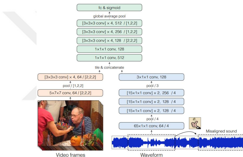
Figure 1: Proposed neural network model by Owens and Efros (2018). Using a fused multisensory representation, they state that a video signal's visual and audio components should be modeled jointly.
