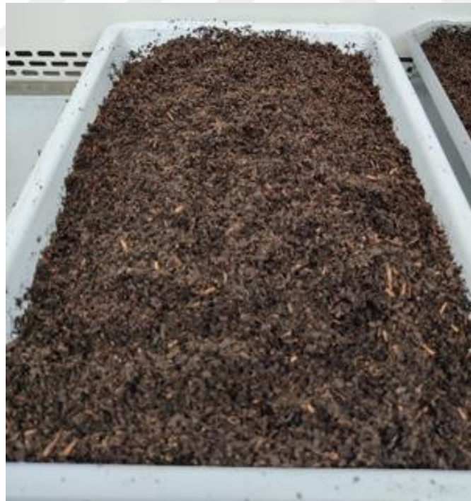
Figure 4. The mixture of Hazelnut husk compost and Bacillus megaterium var. phosphaticum after incubation
