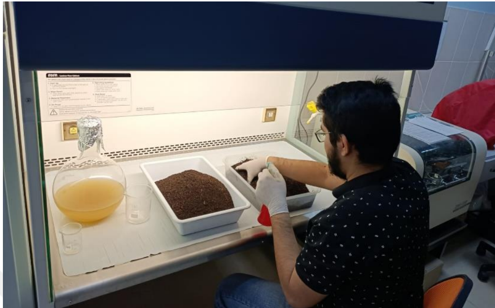
Figure 3. Mixing Bacillus megaterium var. phosphaticum inoculant suspension with the hazelnut husk compost under laminar airflow
