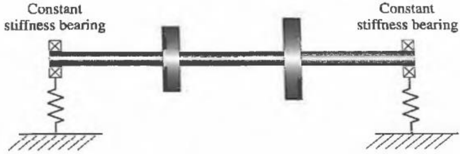
Figure 49: Illustration of two-disk, two bearing rotor [31]
