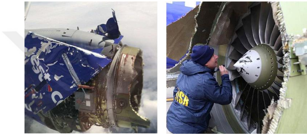
Figure 11: Example Fan Blade-Out Event on Commercial Turbofan Engine during Flight [12]
