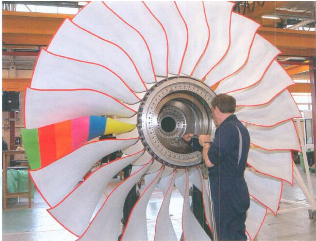
Figure 9: Preparation of Fan Blade-Out Test on Fan Blades [6]
