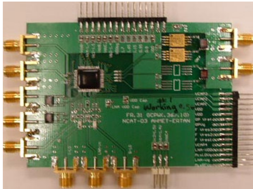
Figure 4.7 Testing board designed for all receiver blocks
