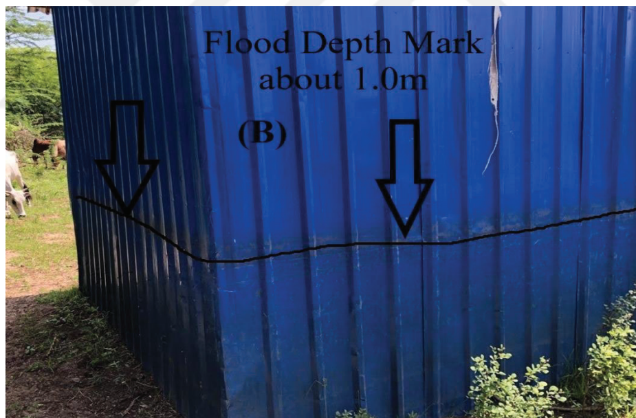
Figure 4.21 (b). The Observed flood depth mark of the Deyr 2019 flood at downstream in the city
