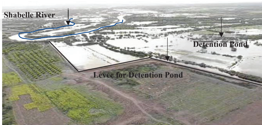
Figure 5.3 (b): Constructed Detention Pond at the upstream in the Left floodplain in the Study Area
