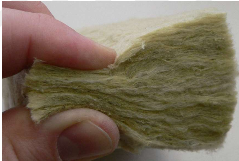
Figure 1.2: Mineral Wool material [1].
