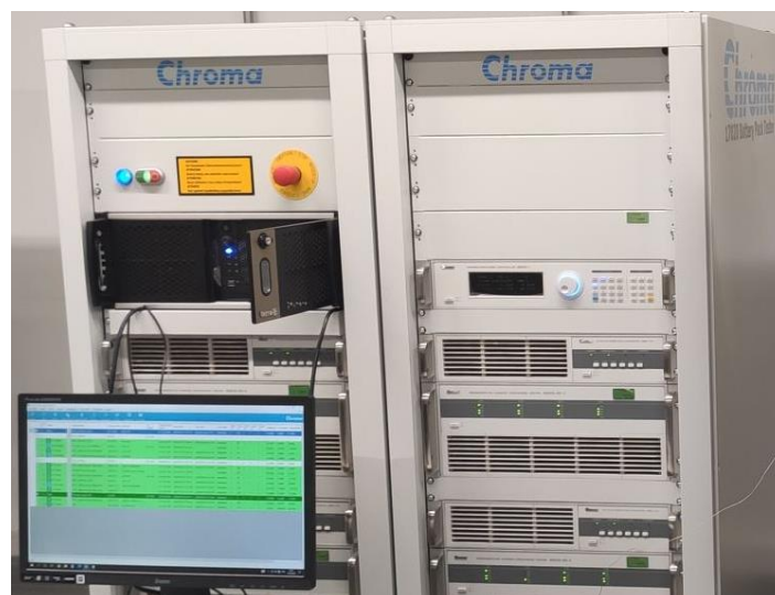
Figure 3.4. Chroma 17020 and 17011 Test Equipment
