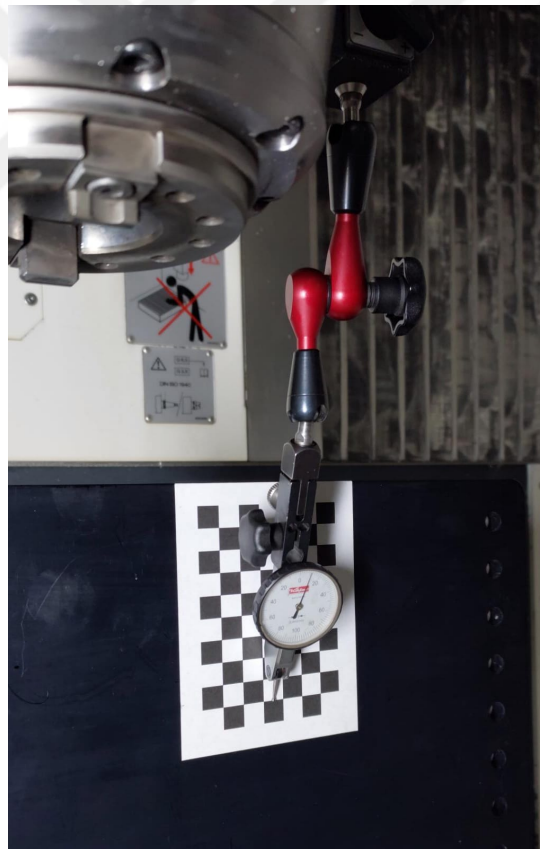
Figure 4.8: The Dial Gauge with Calibration Pattern
