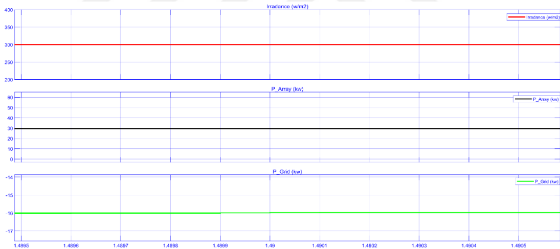
Figure 4.29. The active power from the solar panels and the power grid at 300 \text{ W/m}^2 .
