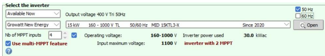
Figure 6.7. Selecting the inverter by PVsyst
