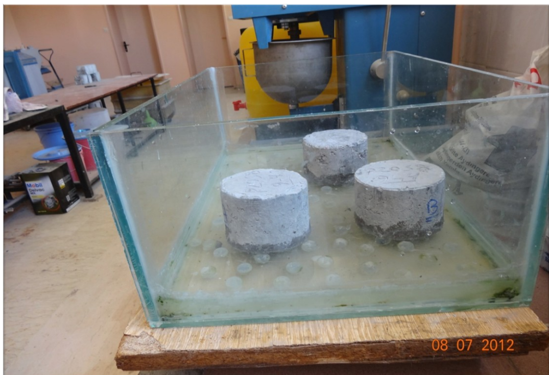
Figure 3.13 Photographic view of sorptivity test
