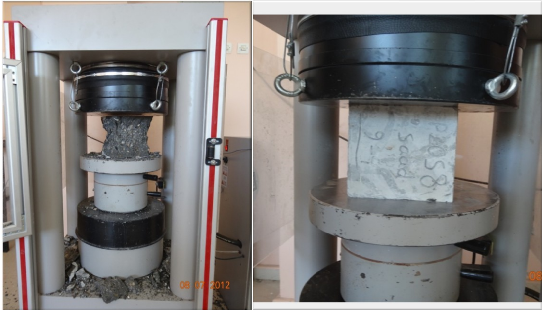
Figure 3.7 Photographic view of compression test
