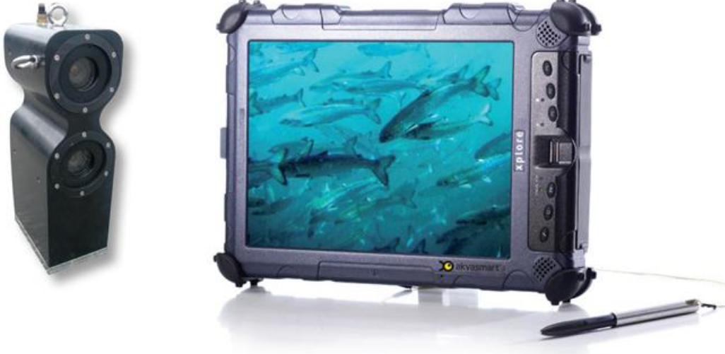
Şekil 3.15 Biyokütle tahmincisi (AkvaGroup, “CameraSystems”, http://www.akvagroup.com/products/cage-farming-aquaculture/camera-systems/biomass-estimator Erişim tarihi 18 Nisan 2012)
