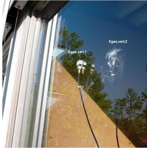
Figure 6.6 : Measurement setup for determining the transmittance of the window glass.
