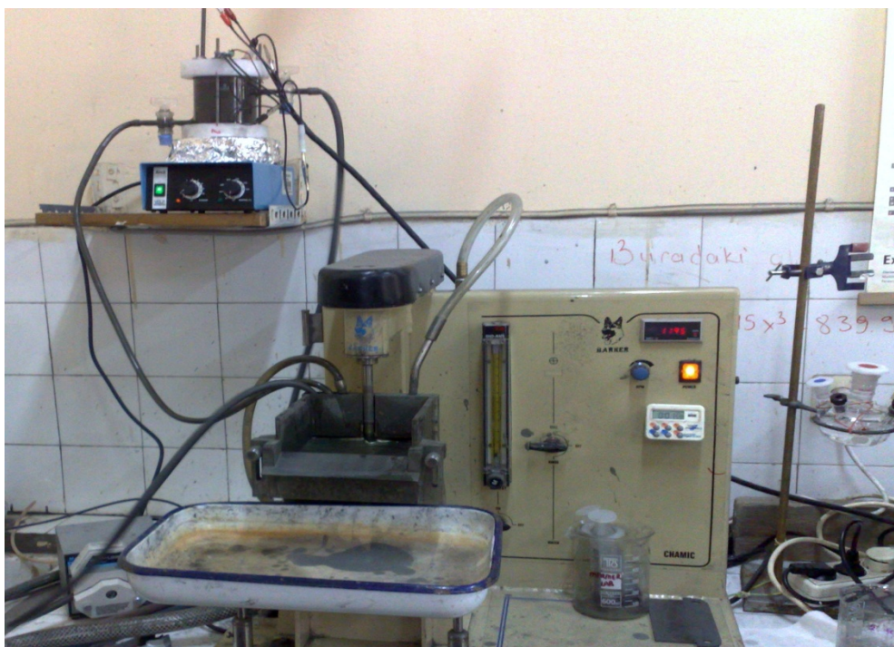
Figure 3.8. Picture of experimental set up of flotation tests
