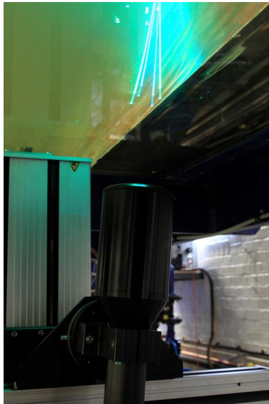
Figure 6.7 : LDV probe with 5^\circ tilt and 45^\circ rotation.
