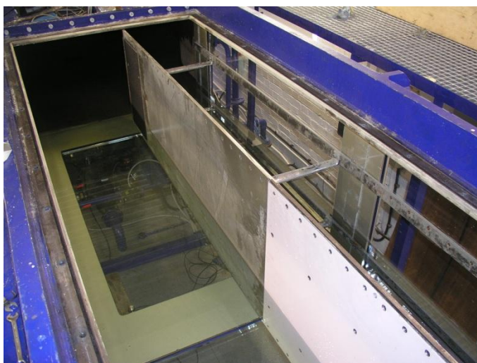
Figure 5.4 : The test plate mounted in the tunnel test section, photograph taken just after the changing of the test specimen (pink coloured).
