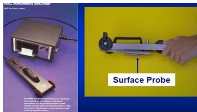
Figure 5.12 : BMT Hull Roughness Analyser.
