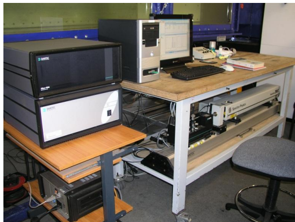
Figure 5.8 : The components of the 2D LDV system
