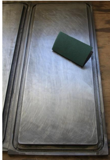
Figure 6.3 : The steel plates were sanded with 120 grid sandpaper before the anti-fouling application.
