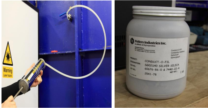
Figure 6.8 : The equipment used for adding seeding to the tunnel water and the seeding material.
