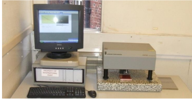
Figure 4.4 : The Omnican Uniscan OSP100A laser profilometer.
