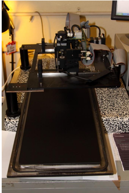
Figure 6.13 : The OSP100 profilometer with the modified legs of the traverse mechanism.
