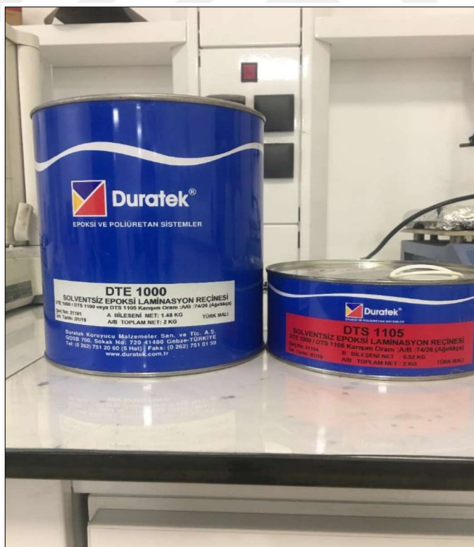
Figure 3.2 Epoxy System Supplied from DURATEK (DTE 1000 is resin (A) and DTS 1105 is slow curing hardener (B)).
