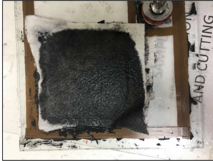
Figure 3.17 Removing the Cured Composite Material from the Mold
