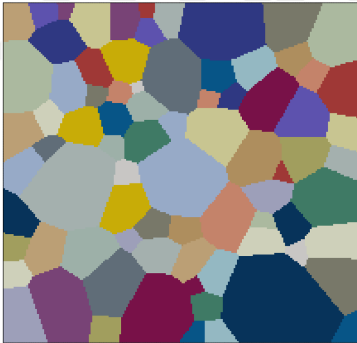
Figure 7.5.2 Grain texture of averaged grain size of 70 micrometers
