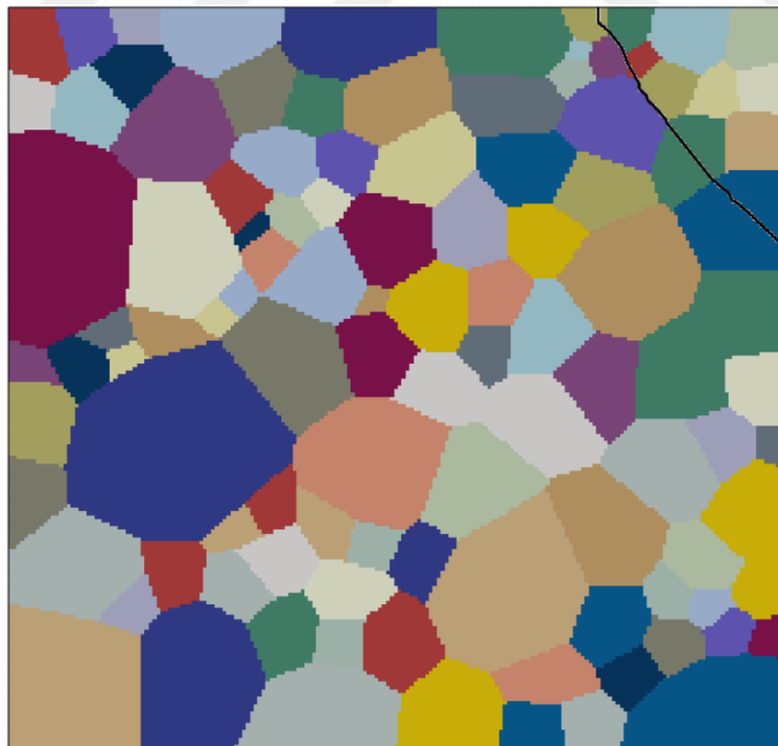
Figure 7.5.4 MAXRSS criterion - crack propagation direction of averaged grain size of 60 micrometers
