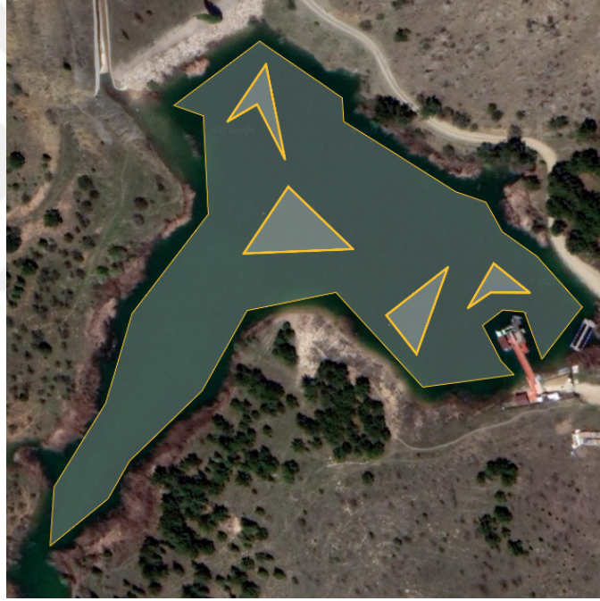
Figure 6.1: Planning arena defined over the dam lake in METU. The orange-edged polygons represent the virtual obstacles that are defined on the map to make the scenarios more challenging.
