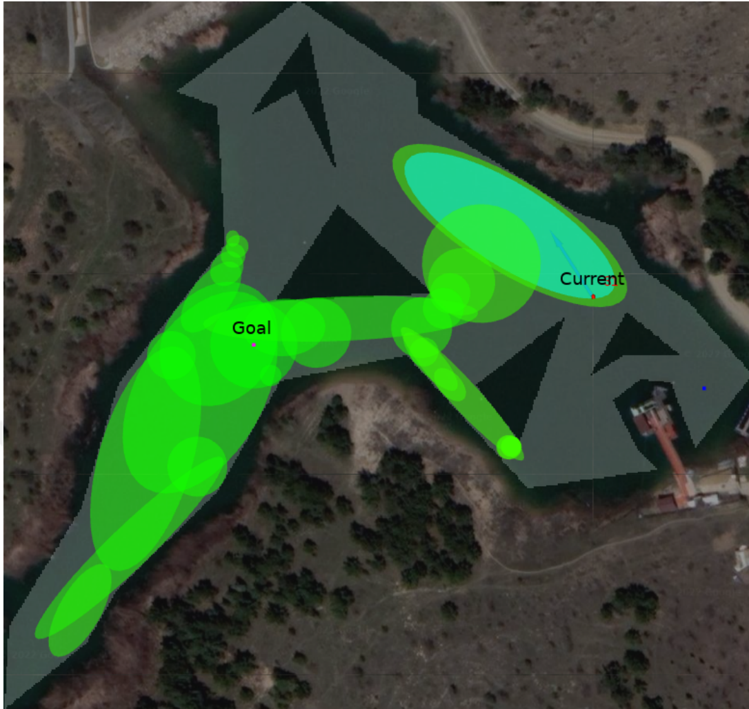
Figure 4.2: Screenshot of RViZ, showing the visualization elements published by the sft_server . In this screenshot, black polygons show the virtual obstacles and green markers show the funnels.
