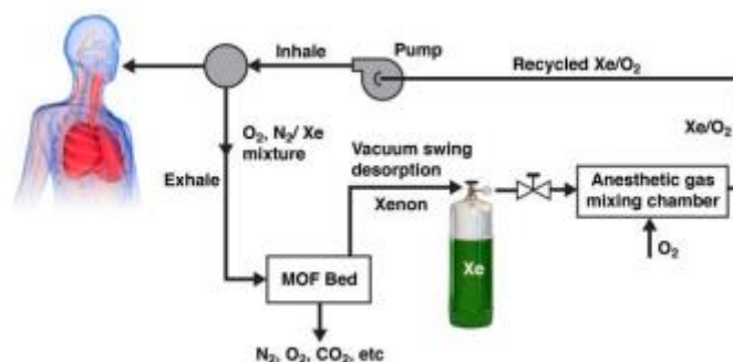
Figure 1.2.2. Schematic representation of the recovery of anesthetic Xe at room temperature using MOFs (Elsaidi et al. 2017).
