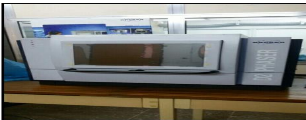
Figure 3.8. X-ray Diffraction Analysis device.
