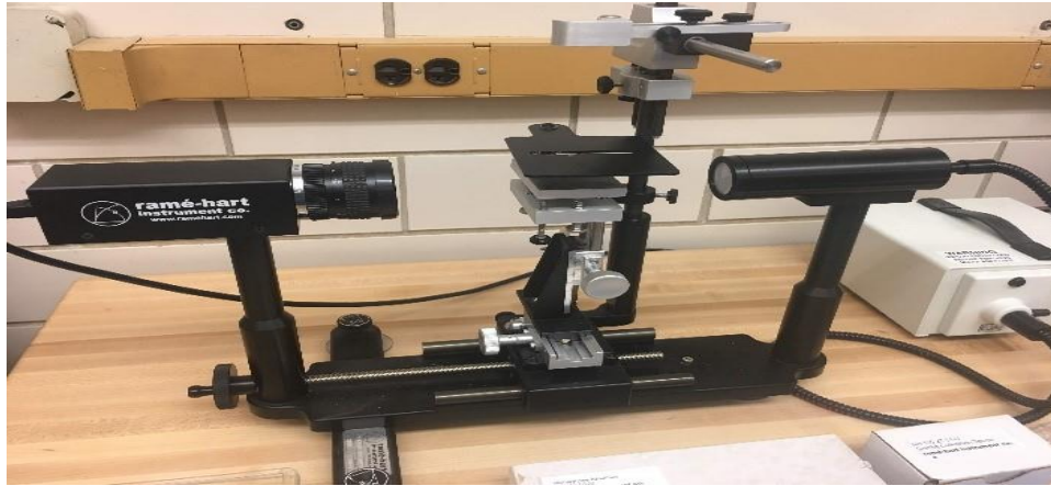
Figure 3.7. Contact angel test device.
