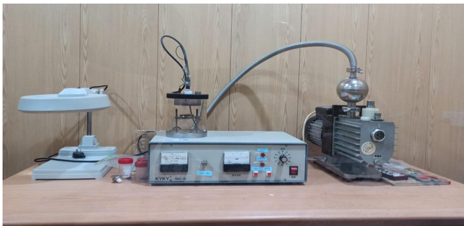
Figure 3.6. Gold coated substrate surface device.
