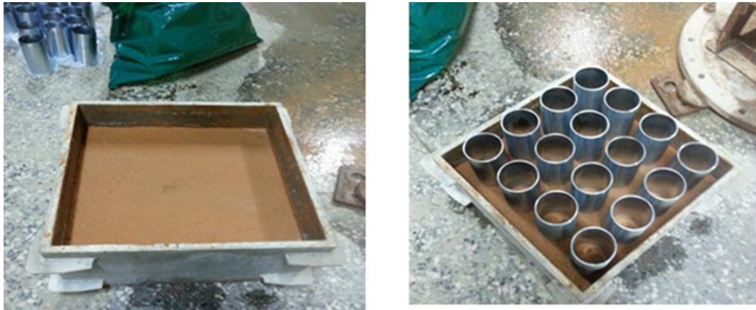
Figure 3.4 a) Ankara clay sample consolidated under 50 kPa vertical stress, b) Specimen samplers
