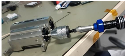
Figure 3.50 : Torquing of fasteners.
