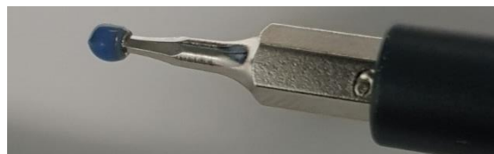
Figure 3.47 : Thread lock applied to a set screw.
