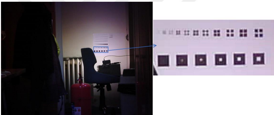
Figure 4.5 : 25mm F4 1443cm – HF25XA-1S @ 1600x1200px – larger detail close up -.
