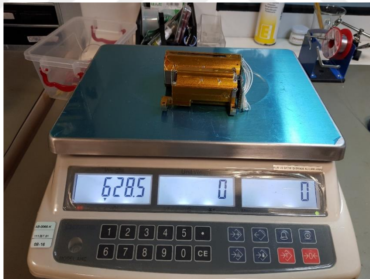
Figure 3.31 : Lenses + sensor boards + structural parts of imaging system.
