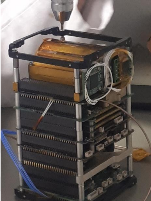
Figure 3.28 : Imaging system integrated to part of the satellite structure.
