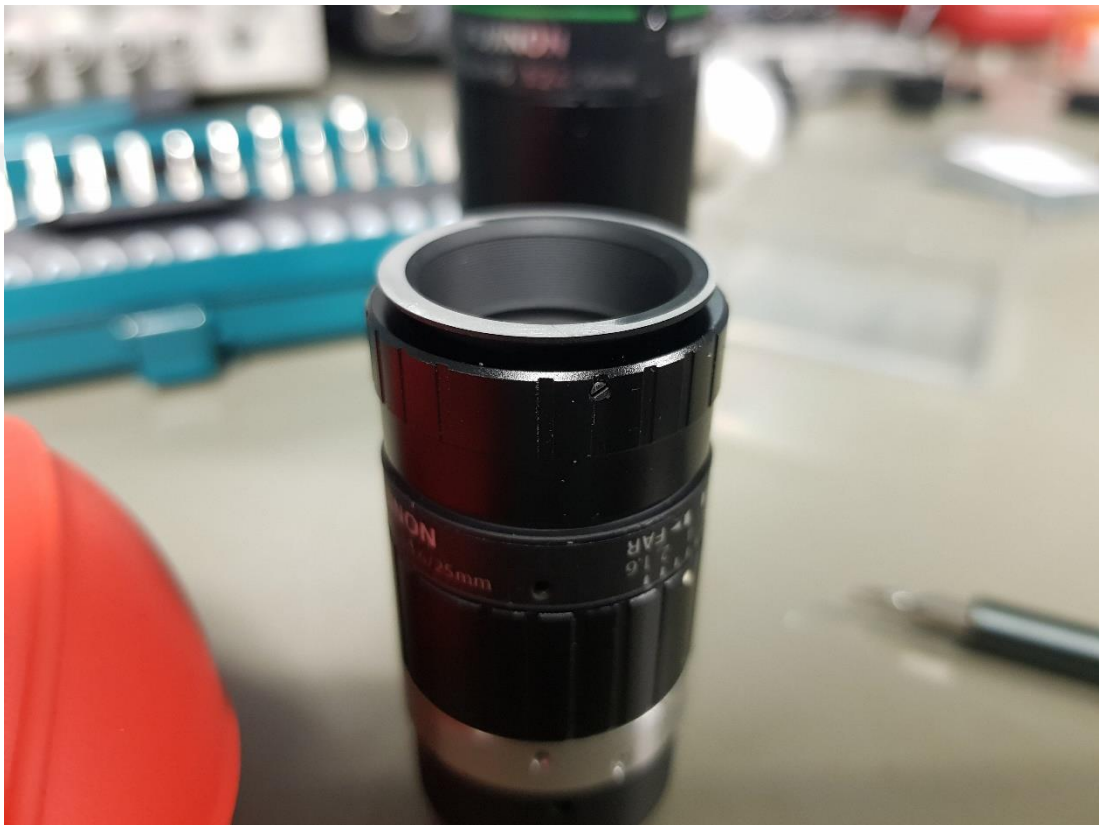
Figure 3.27 : 25mm lens with grounded surface.
