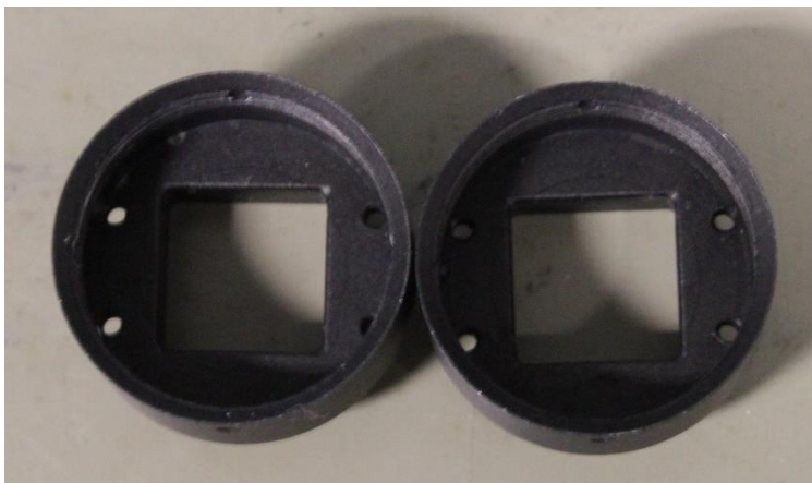
Figure 3.21 : Image of integrated lens mount holder.
