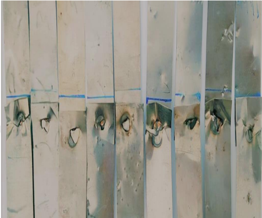
Figure 5.2. Failure specimens after shear test.
