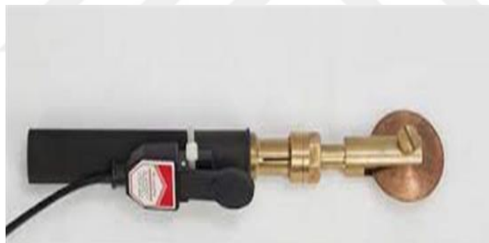
Figure 3.7. Roll spot welding process.
