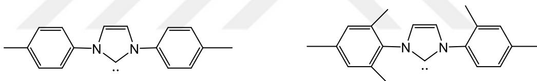
Figure 2.7 Examples of phenyl and mesityl substituted NHCs
