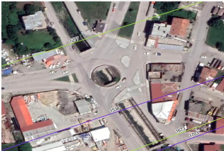
Figure 5.1. View of the bridge (B6) selected as critical one due to past flood events with modelled cross-section numbers (i.e, 1277 and 1538 cross-sections after and before the bridge).
